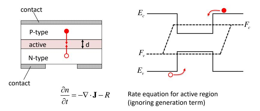
We neglect current spreading in the lateral direction and assume quasi-Fermi level is constant throughout active region.
