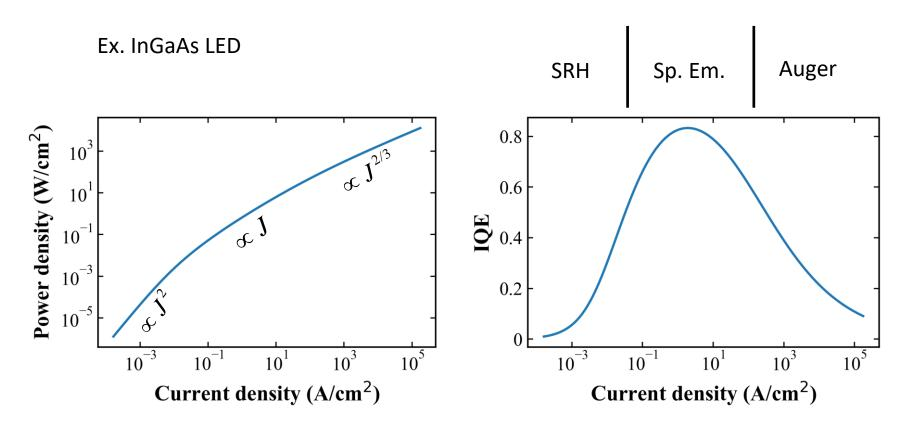
Note: At high current density, other loss mechanisms beside Auger may become important. See for example, controversy surrounding "droop" in GaN LED efficiency at high current.
