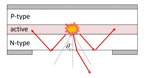
Most emitted light will become trapped in the high-index semiconductor. Only light with angle smaller than critical angle can escape.
