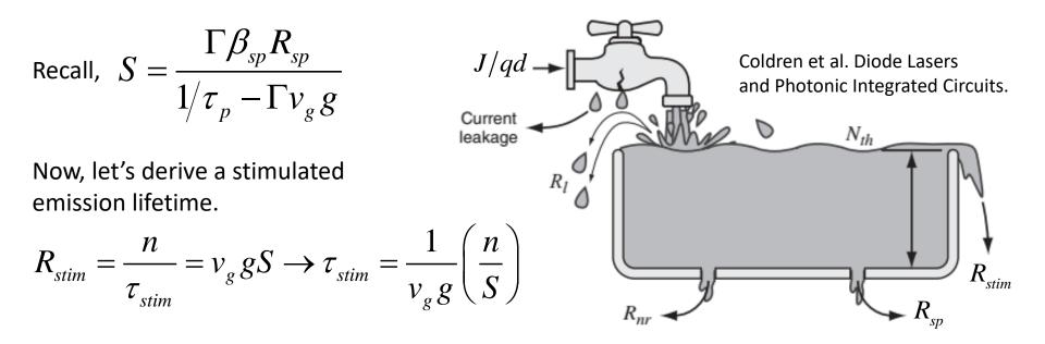
We see that there is a negative feedback loop that does not allow the gain to increase beyond the gain threshold. As current is increased and gain approaches the threshold gain, the photon density increases dramatically thus significantly reducing the stimulated emission lifetime. Any additional current gets immediately "used up" by stimulated emission not allowing the carrier density or gain to increase.
